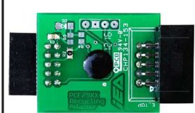
"ZFH-PCF79XX" REMOTE UNLOCKING ADAPTER
